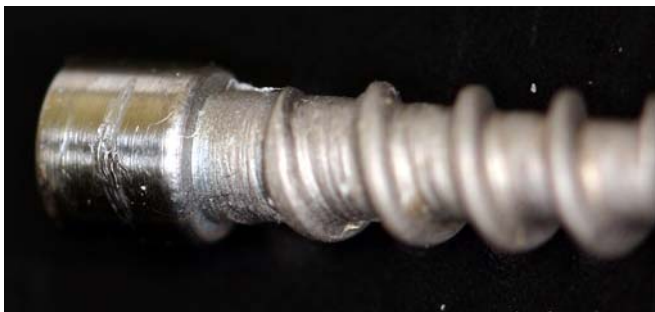
Fig. 1. The damaged titanium implant surface, exaggerates the holding plaque
