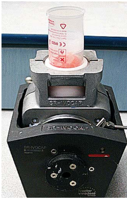
Fig. 3. The polymerisation box locked in the pressure resistant unit
