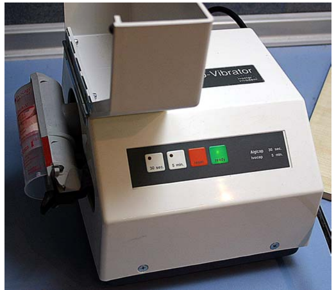
Fig. 4. The mixing unit
