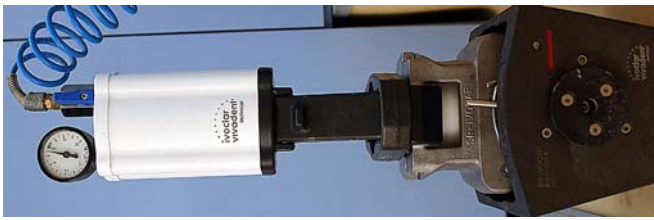
Fig. 5. The IVOCAP prosthesis during the polymerization
